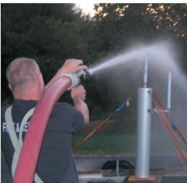
Echomax Active-X-Band RTE being subjected to sustained 75 psi high pressure water jet.
