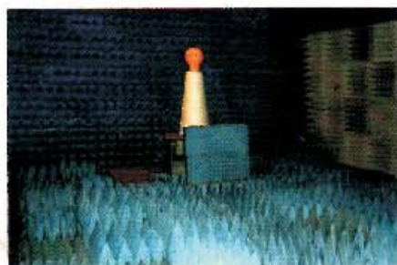
Radar wave-absorbing foam pyramids were used to test the effectiveness of the EM230i at Qinetiq's hi-tech laboratory near Chichester
