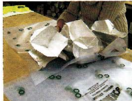
The array inside the EM230's tubing is made from a metalised fabric from DuPont
