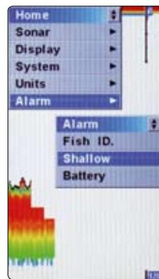
► The Condor 340c has three different alarms that instantly inform you about the fish identification, the shallow water and the battery voltage.
