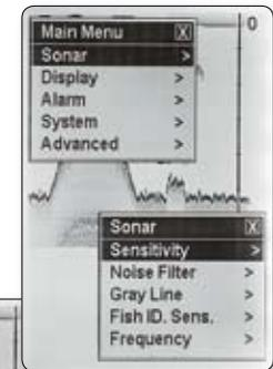
▶ The Noise Filter function reduces the undesired signals that come from your boat engine, turbulence or electrical sources.
