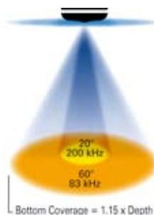
The unit can be either set for single cone operation, large 83 kHz or narrow 200 kHz, at your convenience, or for DualCone scanning, as shown in this image.
